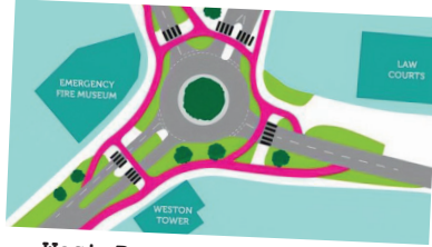
West Bar's "Dutch-style" roundabout will give priority to people walking and cycling - coming soon!
